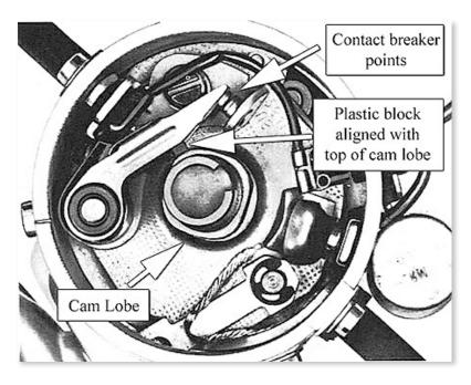
Guessing is not as bad as it might seem. Remember we're trying to make the car run well enough to get home. The engine will tolerate a larger gap more readily than a small one. On the other hand, a gap equivalent to a credit card thickness is too wide.
