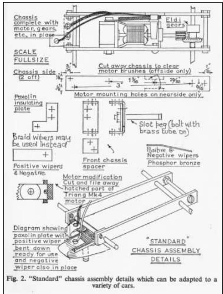
Fig. 2. "Standard" chassis assembly details which can be adapted to a variety of cars.
